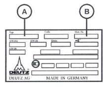
The model type A and the engine serial No. B are given in the engine identification plate.
