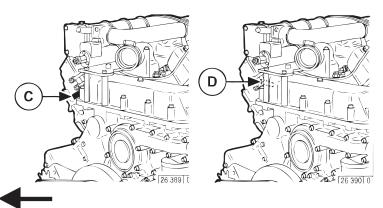
The engine identification plate C is mounted to the crankcase.
