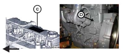
The engine identification plate C is mounted to the valve covering hood. The serial No. D is also stamped into the crankcase.
