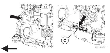
The engine identification plate is mounted to the crankcase.
