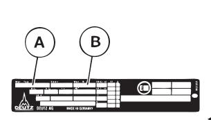
The model type A and the engine serial No. B are given in the engine identification plate.
