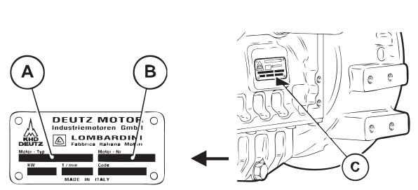
The model type A and the engine serial No. B are given in the engine identification plate.
