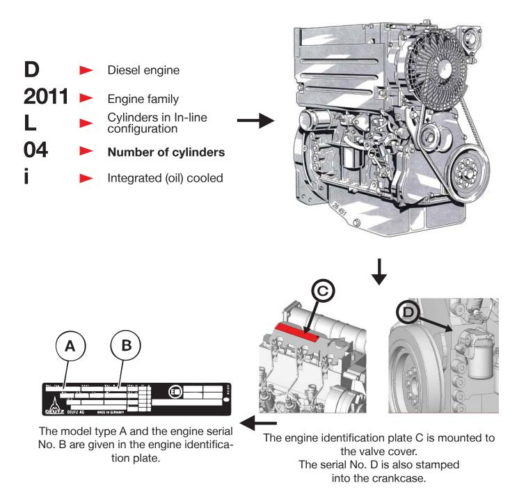
For integrated cooled engines with air discharge duct the engine identification plate is located between cooling blower housing and air duct.
