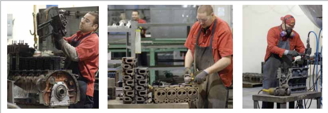
AREA 2: All parts are disassembled and cleaned rigorously
